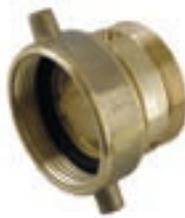
Female NH to male BSP reducer (swivel), are available in nominal sizes 1 ½"- 4" Swivel system adapters are always delivered with Pin Lug.
