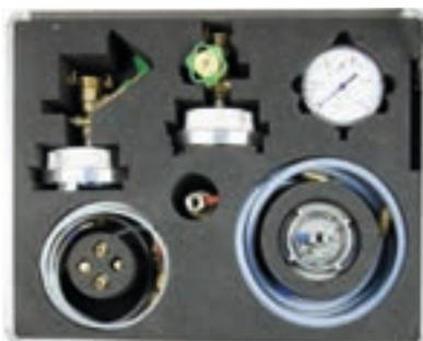
The test case set 199797A enables backflow preventer to be tested in addition to testing B-FW and BA. The Backflow preventer BA has a test connection from 1/4" female BSP thread.
