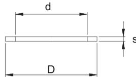
All Storz, GOST, BS and NOR couplings with BSP female thread, are equipped with a flat seal. Aluminum and brass couplings always have a NBR seal. Depending on the application, our stainless steel couplings have either a flat Viton or EPDM seal.
