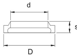
Only BS female threads are equipped with seal.
