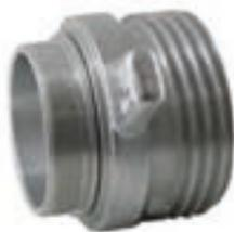
The double thread nipple is supplied with a 5 1/2" DIN 11 thread inlet and a 4" BSP thread outlet.
