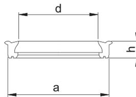
The Storz sealing rings are available in different materials, depending on the application. The most used seals are NBR, EPDM, silicone and Viton. The delivery/suction seals have an external lip.
