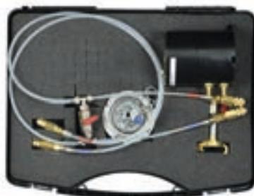
The plastic test cases, are used to store all necessary parts in order to perform the audit of the backflow preventer BA.
