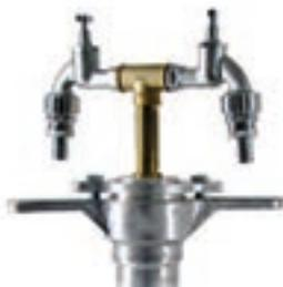
The standpipes are designed for hoses up to 1". We provide standpipes with outflow valve with 3/4 tap. Upon request, we can deliver all with DN 40 claw couplings or Storz D-25 fixed couplings. Not for drinking water.
