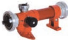
Inductors are installed between the pump and foam tubes and can be used both with medium foam nozzle but also with heavy foam nozzle. The foam inlet of each inductor is always equipped with a Storz D-25 aluminum coupling.
