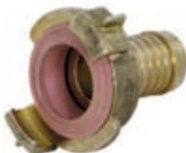
These claw couplings are used for drinking water hoses up to 1". The tail piece is serrated. The binding is usually done using hose clamps. The quick couplings type „P“ can be coupled with GEKA systems.
