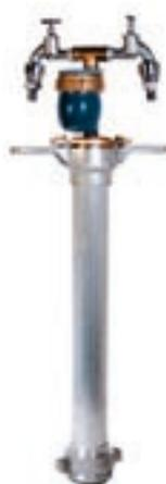
On a swivel standpipe head with taps, you can connect hoses which have the following sizes ¾ or 1". We offer our standpipes with tap and ¾" hose tail. Our standpipes are equipped with water meters Q<sub>3</sub> 4. These is located on the head of the standpipe. Not for drinking water.
