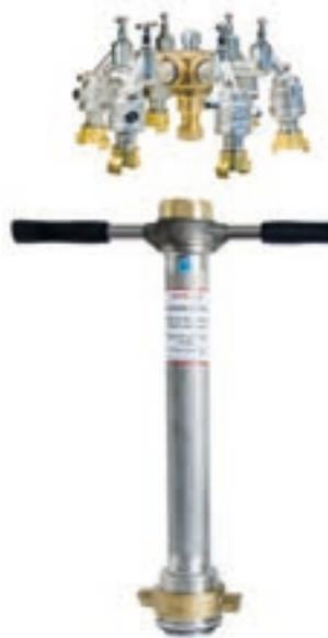
The Light version standpipes have a 2" pipe and a rotatable head part. Matching water meters can be provided or integrated. By these standpipes, the individual approval is given according to EN 1717.
