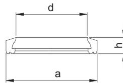
The Storz sealing rings are available in different materials, depending on the application. The most used seals are NBR, EPDM, silicone and Viton. The delivery seals are flat.
