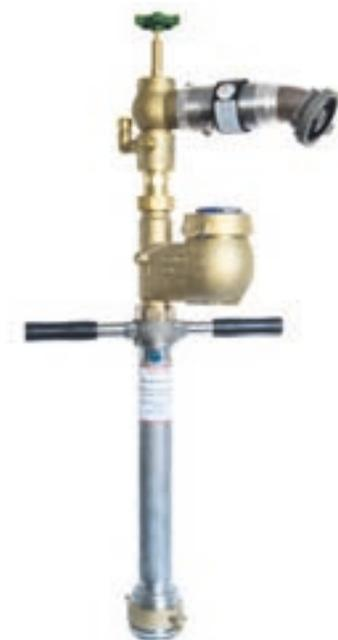
The Light version standpipes have a 2" pipe and a rotatable head part. With this version, the handles can be screwed in. These standpipes can also be provided with up to 2 drain valves with BA backflow preventers and claw adapters, in addition to the Storz C-52 coupling.
