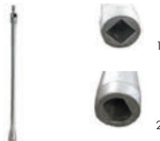
For the British underground hydrants there are two versions of standpipe keys. The type A version refers to a square form and the type B version to an oval form. The standpipe key is manufactured in aluminum and on request it can be produced in special lengths.
