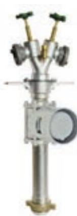
The flow rate can be recorded during the flushing process with these standpipes. They can also be used to measure the flow rate in m<sup>3</sup>/h. Free flow and low pressure loss thanks to MID water meter.  $Q_4$  125m<sup>3</sup>/h, continuous load  $Q_3$  100 m<sup>3</sup>/h.
