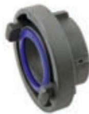
By default, adapters are provided with a delivery seal. If required, we can also provide a delivery/suction seal. All adapters are equipped with a flat seal inside the female thread.
