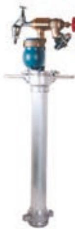
The standpipes have 1x Storz C-52 and additionally in option a tap as connector. Our standpipes are equipped with the water meters Q<sub>3</sub> 4 or Q<sub>3</sub> 10. Not for drinking water.
