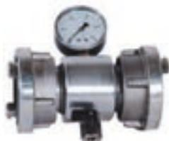
Pressure measuring instrument with a range from 0 to 25 bar. Inlet and outlet with swivel Storz couplings.
