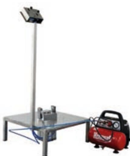
The inspection system was developed to inspect the functionality of the water meters on standpipes with pressurised air. The standpipe is pneumatically fixated.
